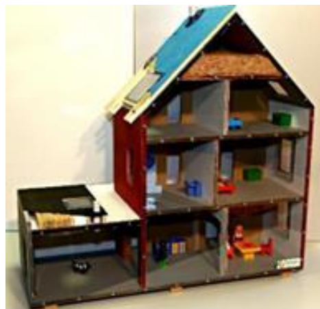
Figure 10. Example of a pedagogical tool that illustrates the effect of airtightness on the mechanical ventilation by running a smoke generator
